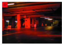
Photographs 1-6 show car park clearing after being fully smoke logged
